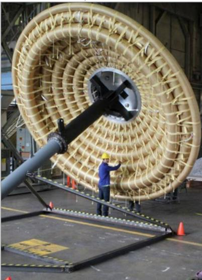
The inflatable structure is a series of rings made of braided Kevlar that are stacked together. Credit: NASA
