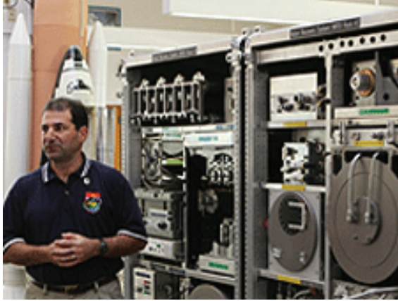
Figure 1. NASA scientist Bob Badigan in front of the Water Recovery System used on the ISS. Image credit: NASA
