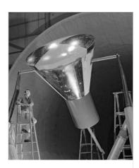
Mercury capsule model in the Langley Full-Scale Tunnel, January 1959. Credit: NASA
