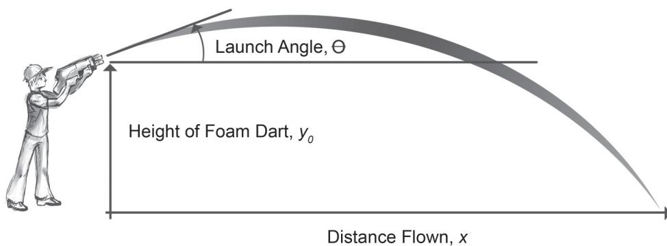
Figure 2: Launch set-up.
