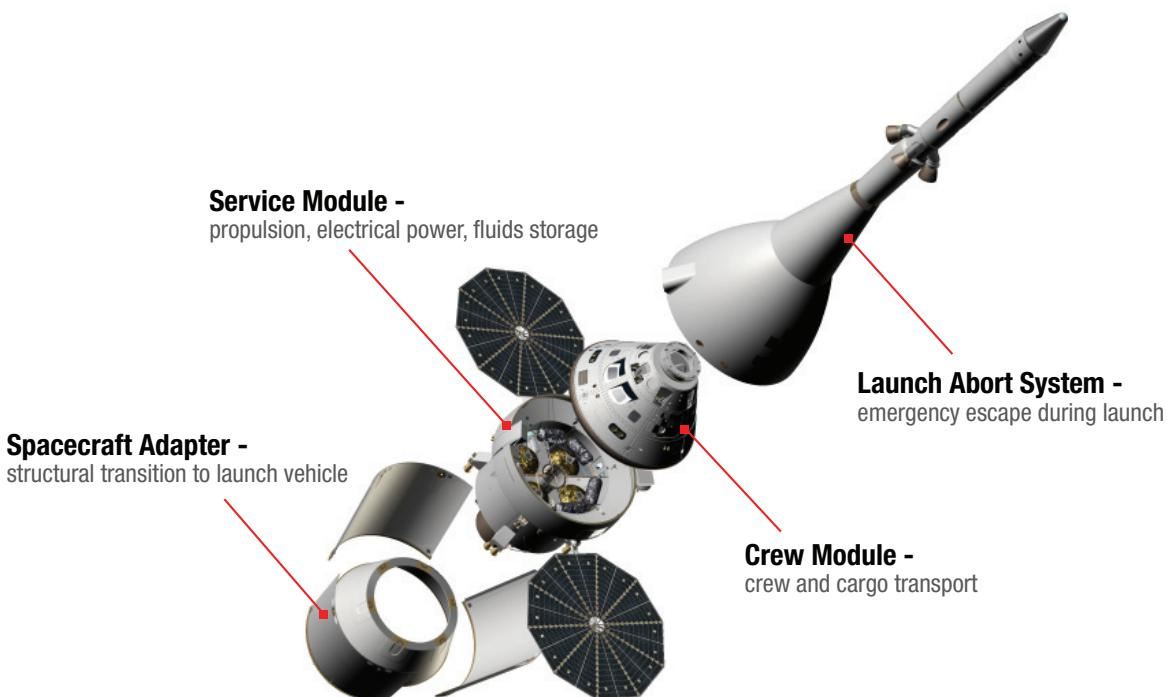
Figure 1: Components of the Orion spacecraft. Image Credit: NASA
