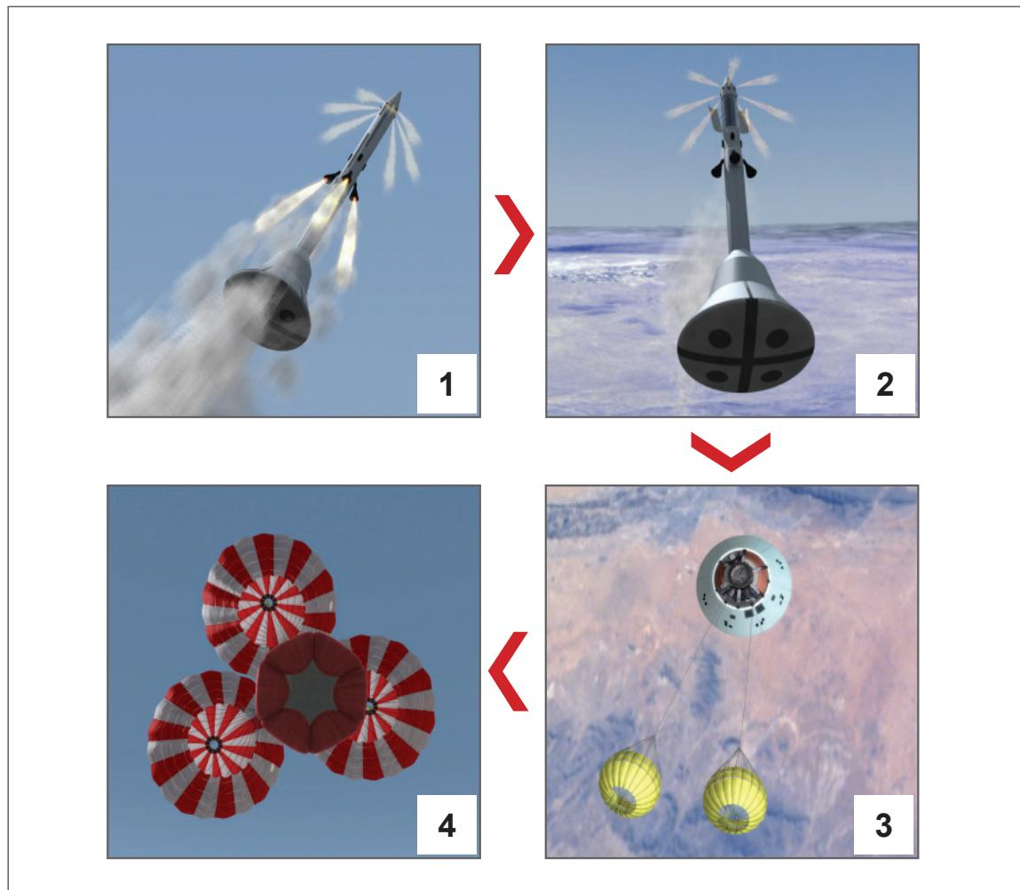
**Figure 2:** Orion's launch abort system is designed to pull the crew module to safety in an emergency.
