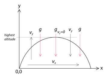
Figure 1. Parabolic motion of a projectile.
