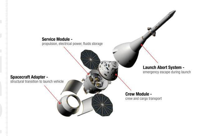
Figure 1: Components of the Orion spacecraft. Image Credit: NASA
