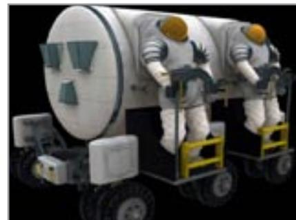
Figure 1: Concept of one potential design for a future lunar rover. Spacesuits would be attached to the exterior of the rover. **Image Credit:** NASA
