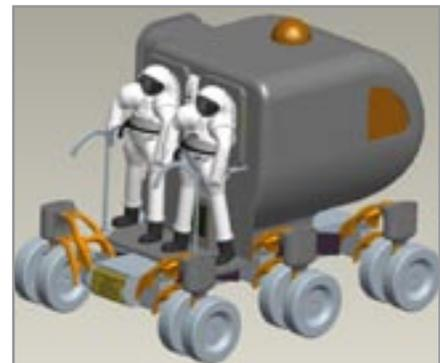
Figure 2: Concept of one potential design for a future lunar rover. Spacesuits would be attached to the exterior of the rover. **Image Credit:** NASA
