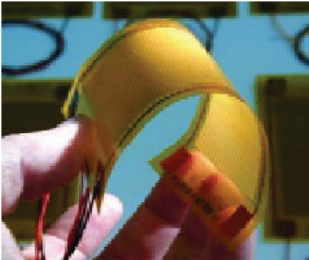
Figure 2. This piezoelectric material, developed at NASA's Langley Research Center (LaRC), can "feel" deformations such as bending or surface pressure, producing a small voltage in response that can act as a signal for a central computer.
