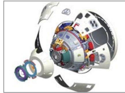
Figure 1: Exploded view of Orion.
