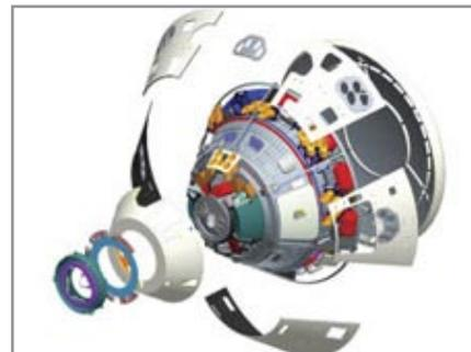
Figure 1: Exploded view of Orion.
